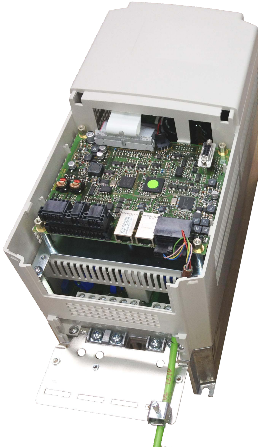
Strain relief at housing G by use of mounting kit G0F4T88-0004
