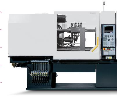
KEB provides the right solutions for all types of injection moulding machines: from fully electric machines to hybrid machines (electric and servo-hydraulic) to hydraulic machines for which appropriate servo pump software is available. Fully electric solutions with non-linear torque control are ideal for regulating the clamping unit and thus reducing the machine cycle.
